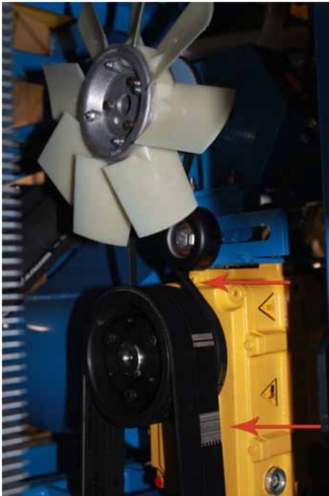
Blower to Pump Belt
