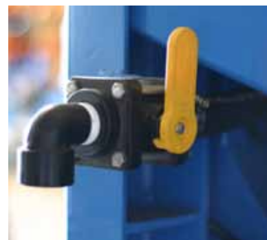
The Main Tank Dump Valve
